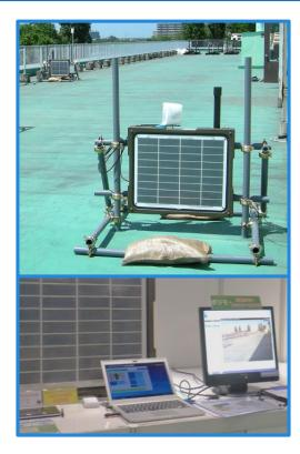
Weather measurement device was connected to a Poggimo on a rooftop
